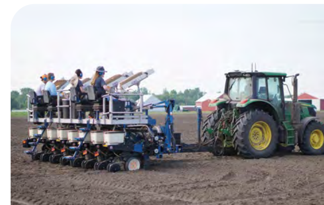
One of eight labs running experiments at the Field Site using a GPS-enabled precision planter.
